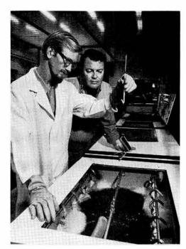
UNDER DIRECTION of supervisor Shary Holmes (4222-5), right, John Arnold immerses a piece part into plating tank to perform nickel plating.
